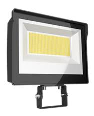
Ultra-economy field adjustable X17 is available in three sizes and a total of 6 lumen packages, all with a wide  $7H \times 7V$  NEMA distribution that makes them the optimal floodlight for a large variety of general-purpose applications. 0-10V dimming is standard on all models.
