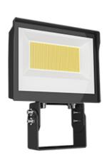
Ultra-economy field adjustable X17 is available in three sizes and a total of 6 lumen packages, all with a wide 7H x 7V NEMA distribution that makes them the optimal floodlight for a large variety of general-purpose applications. 0-10V dimming is standard on all models.
