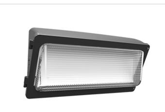
**Project:** Type: Prepared By: Date: LED Info **Driver Info** Constant Watts 130/100/65W Туре 120V N/A Color Temp 3000/4000/5000K 208V N/A Color Accuracy 82-86 CRI 240V N/A L70 Lifespan 100,000 Hours 277V N/A Lumens 9,946-18,809 lm
