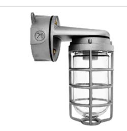
Die cast aluminum construction. Wall bracket plus junction box with sturdy mounting lugs. Medium base socket, 1/2" or 3/4" NPS hub size and a variety of globes. incandescent lamp A21 for 100 series, PS25 for 200 Series. Lamp not supplied.
