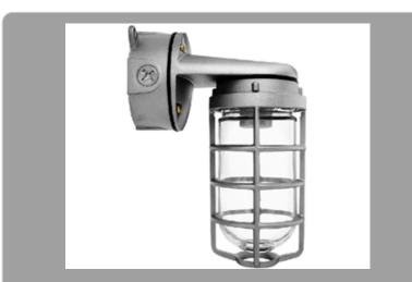
Die cast aluminum construction. Wall bracket plus junction box with sturdy mounting lugs Medium base socket, 1/2" or 3/4" NPS hub size and a variety of globes. incandescent lamp A21 for 100 series, PS25 for 200 Series. Lamp not supplied.
