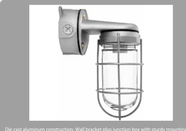
Die cast aluminum construction. Wall bracket plus junction box with sturdy mounting lugs Medium base socket, 1/2" or 3/4" NPS hub size and a variety of globes. incandescent lamp A21 for 100 series, PS25 for 200 Series. Lamp not supplied.
