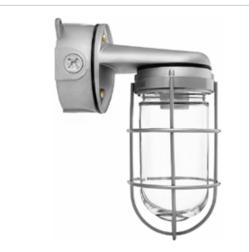
Die cast aluminum construction. Wall bracket plus junction box with sturdy mounting lugs. Medium base socket, 1/2" or 3/4" NPS hub size and a variety of globes. incandescent lamp A21 for 100 series, PS25 for 200 Series. Lamp not supplied.
