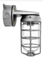
Die cast aluminum construction. Wall bracket plus junction box with sturdy mounting lugs. Medium base socket, 1/2" or 3/4" NPS hub size and a variety of globes. incandescent lamp A21 for 100 series, PS25 for 200 Series. Lamp not supplied.
