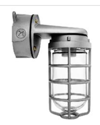
Die cast aluminum construction. Wall bracket plus junction box with sturdy mounting lugs. Medium base socket, 1/2" or 3/4" NPS hub size and a variety of globes. incandescent lamp A21 for 100 series, PS25 for 200 Series. Lamp not supplied.
