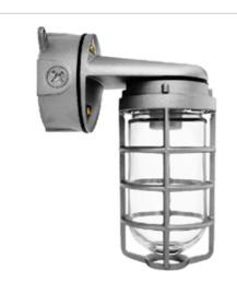
Die cast aluminum construction. Wall bracket plus junction box with sturdy mounting lugs. Medium base socket, 1/2" or 3/4" NPS hub size and a variety of globes. incandescent lamp A21 for 100 series, PS25 for 200 Series. Lamp not supplied.
