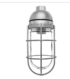
Pendant mount, die cast aluminum construction. Medium base socket, 1/2" or 3/4" NPS pendant thread and a variety of globes. incandescent lamp A21 for 100 Series, PS25 for 200 Series. Lamp not supplied.
