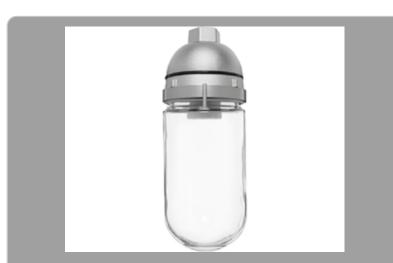
Pendant mount, die cast aluminum construction. Medium base socket, 1/2" or 3/4" NPS pendant thread and a variety of globes. incandescent lamp A21 for 100 Series, PS25 for 20 Series. Lamp not supplied.
