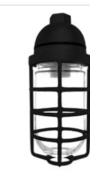
Pendant mount, die cast aluminum construction. Medium base socket, 1/2" or 3/4" NPS pendant thread and a variety of globes. incandescent lamp A21 for 100 Series, PS25 for 200 Series. Lamp not supplied.
