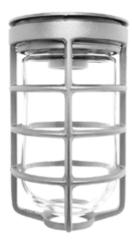
Die cast aluminum construction. Mounts to existing surface or recessed 4" boxes. Adapter plate provided. Medium base socket and a variety of globes. incandescent lamp A21 for 100 Series, PS25 for 200 series. Lamp not supplied.
