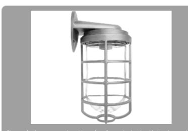
Die cast aluminum construction with sturdy wall mounting bracket. Medium base socket and a variety of globes. incandescent lamp A21 for 100 Series, PS25 for 200 Series. Lamp not supplied.
