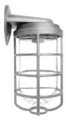
Die cast aluminum construction with sturdy wall mounting bracket. Medium base socket and a variety of globes. incandescent lamp A21 for 100 Series, PS25 for 200 Series. Lamp not supplied.
