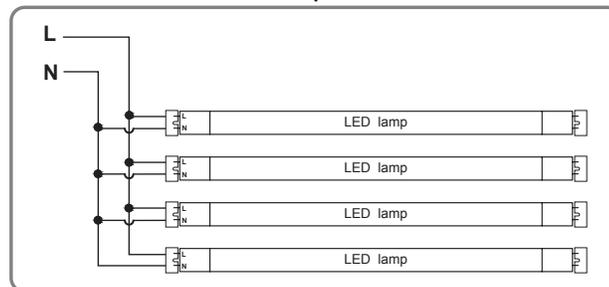
The below ballast wiring represents typical configuration. The actual ballast wiring varies according to ballast model. It is not needed to change socket (if in good condition) to operate double ended lamps, regardless the type of sockets. Please make sure one side of fixture is connected to Live (L) and the other side to Neutral (N).
