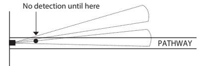
**Solution:** "Micro Adjust" sensor by moving sideways 1/4". This may move the zones to allow earlier detection.
