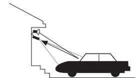
**Solution:** Aim sensor away from reflective objects or move the objects lower and reduce sensitivity.
