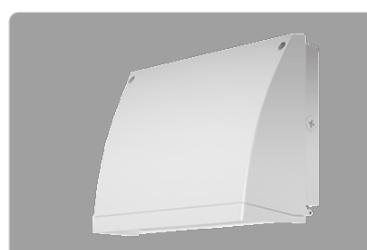
37, 57 and 62 Watt SLIM Wall packs are designed to cover the footprint of most traditional wall packs. They are suitable for mounting heights from 20' to 30', and replace HID Wattages from 200W MH to 320W MH. These ultra-high efficiency fixtures are available in cutoff or full cutoff models.
