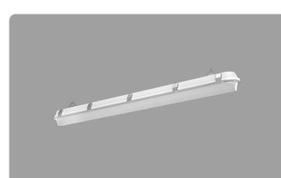
The four-foot SHARK is available in 36W and 50W versions. This impact-resistant linear LED washdown fixture is ideal for tunnels, stairwells and other hard-to-reach areas where relamping is difficult and costly. 0-10V dimming models available.
