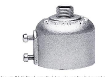
Aluminum Pole Slipfitters for mounting fixtures or boxes to top of poles or posts. 1/2" top tap standard. 3/4" top tap on R5-3/4 and R7-3/4 only. Set screws provided.
