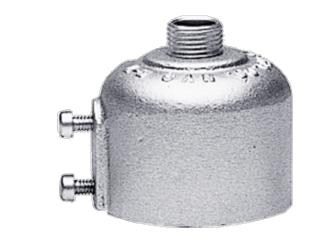
Aluminum Pole Slipfitters for mounting fixtures or boxes to top of poles or posts. 1/2" top tap standard. 3/4" top tap on R5-3/4 and R7-3/4 only. Set screws provided.
