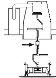
5. Carefully route wires into fixture housing. Push the retrofit kit and metal friction clips into the housing. (Fig. 5)
