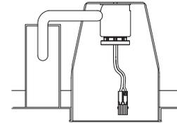
3. Select desired color temperature (CCT) level using switch on driver box. (Fig. 3)
