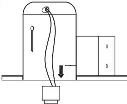
4. Screw the E26 adapter into the socket inside the housing. (Fig. 9)
