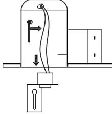
3. Remove existing socket mounting plate from the recessed housing and then remove lamp socket from the plate. (Fig. 8)
