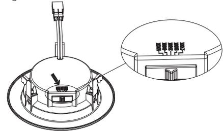
4. Plug E26 base cable connection into the recessed retrofit kit. (Fig. 4)
