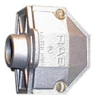
Die cast aluminum for thru-wall or conduit end floodlight mounting. Three 1/2" threaded holes. Side opening cover for easy access and splicing. 1/2" thru wall tapped hub.
