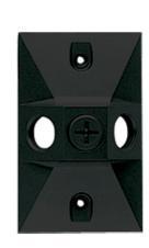
Die cast rectangular covers with one or three 1/2" threaded holes. Fits FS, cast and recessed single outlet boxes. Supplied with thick foam rubber gasket and two #6-32 stainless steel screws. 3 hole cover comes with one die cast 1/2" close-up plug.
