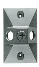
Die cast rectangular covers with one or three 1/2" threaded holes. Fits FS, cast and recessed single outlet boxes. Supplied with thick foam rubber gasket and two #6-32 stainless steel screws. 3 hole cover comes with one die cast 1/2" close-up plug.
