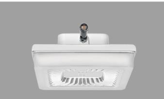
This ultra high efficiency LED garage light delivers up to 118 lumens per Watt. An integrated motion/photo sensor option provides multi-level lighting control. Available in 30, 42 and 55 Watt versions that replace 70 to 175 Watt metal halide fixtures. Fixture measures 14" L x 14" W.
