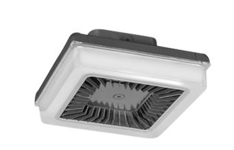
This ultra high efficiency LED garage light delivers up to 118 lumens per Watt. Available in 30, 42 and 55 Watt versions that replace 70 to 175 Watt metal halide fixtures. Fixture measures 14" L x 14" W.
