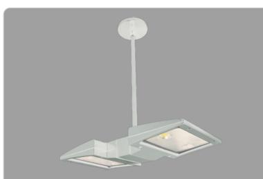
The PLED is a high performance LED downlight available in 52, 40, 26 and 20W versions in both Cool and Warm Color Temperatures. Pendant mount with hang-straight and 6", 12" and 18" stems included. Stems can be combined up to 36" max length.
