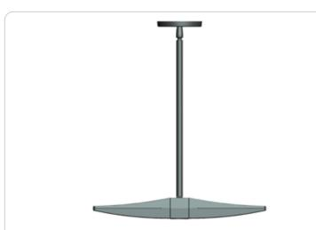
The PLED is a high performance LED uplight available in 52, 40, 26 and 20W versions in both Cool and Warm Color Temperatures. Pendant mount with hang-straight and 6", 12" and 18" stems included. Stems can be combined up to 36" max length.
