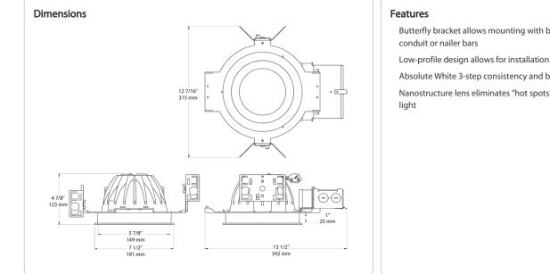
Butterfly bracket allows mounting with bar stock, "C" channel, 1/2"
