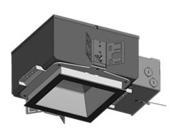
Easy to install 6" rough-in with die-cast aperture ring, removable driver, thermal protector and adjustable butterfly brackets. This rough-in is designed to make new construction recessed downlighting easy .
