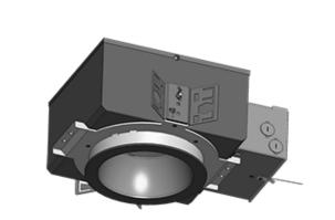
Easy to install 6" rough-in with die-cast aperture ring, removable driver, thermal protector and adjustable butterfly brackets. This rough-in is designed to make new construction recessed downlighting easy.
