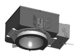
Easy to install 6" rough-in with die-cast aperture ring, removable driver, thermal protector and adjustable butterfly brackets. This rough-in is designed to make new construction recessed downlighting easy .
