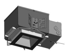
Easy to install 4" rough-in with die-cast aperture ring, removable driver, thermal protector and adjustable butterfly brackets. This rough-in is designed to make new construction recessed downlighting easy .
