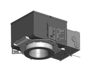
Easy to install 4" rough-in with die-cast aperture ring, removable driver, thermal protector and adjustable butterfly brackets. This rough-in is designed to make new construction recessed downlighting easy.
