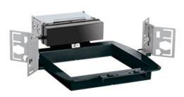
Easy to install 4" rough-in with die-cast aperture ring, removable driver, thermal protector and adjustable butterfly brackets. This rough-in is designed to make new construction recessed downlighting easy .
