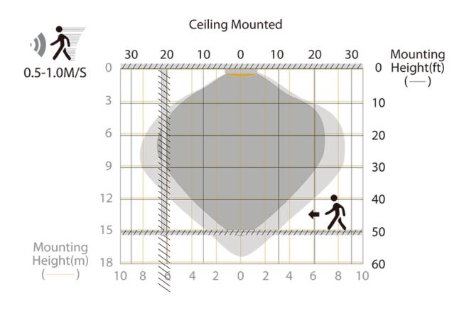
Highest mounting height is: MVS20x/LCB: 6m/20ft, MVS50x/LCB: 15m/49ft This gure indicates the maximum distance at the highest mounting height with 100% sensitivity.
