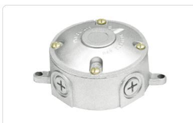
Die cast aluminum wiring box with weatherproof gasket, ground screw, and two sturdy lugs for wall or ceiling mounting. Die cast aluminum cover without center hole supplied with 4 stainless steel screws.
