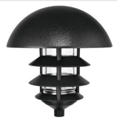
New! 4 Tier Dome Top offers wide light spread for wider walkways and parking lots where maximum light is required. Rugged die cast aluminum housings. Threaded, gasketed clear glass globe for durable weatherproofing and easy relamping. 1" long, 1/2" threaded nipple included for easy mounting. 75 Watt max. incandescent, 13 Watt fluorescent.
