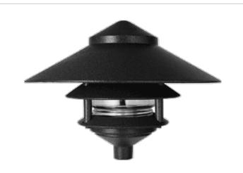
Rugged die cast aluminum 6" diameter housings. Threaded, gasketed clear glass globe for durable weatherproofing and easy relamping. 1" long, 1/2" threaded nipple included for easy mounting. 75 Watt max.
