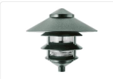
Rugged die cast aluminum 6" diameter housings. Threaded, gasketed clear glass globe for durable weatherproofing and easy relamping. 1" long, 1/2" threaded nipple included for easy mounting. 100 Watt max.
