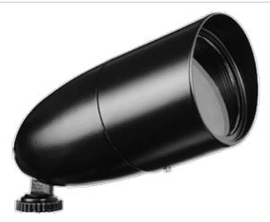
PAR16 floodlight with die cast aluminum housing, integral glare shield and tempered lens. Sleek good looks with minimal size. Supplied with 6" leads and ground wire. Medium base PAR16 lamp, 60 Watt max. Lamp not supplied.
