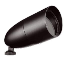
PAR16 floodlight with die cast aluminum housing, integral glare shield and tempered lens. Sleek good looks with minimal size. Supplied with 6" leads and ground wire. Medium base PAR16 lamp, 60 Watt max. Lamp not supplied.
