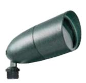
Low voltage MR16 flood with die cast aluminum housing, integral glare shield and tempered lens. Sleek good looks with minimal size. Supplied with 36" SPT-1 cord for installation on low voltage systems. MR16 lamp, 50 Watt max. Lamp not supplied.
