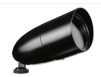
Low voltage MR16 flood with die cast aluminum housing, integral glare shield and tempered lens. Sleek good looks with minimal size. Supplied with 36" SPT-1 cord for installation on low voltage systems. MR16 lamp, 50 Watt max. Lamp not supplied.
