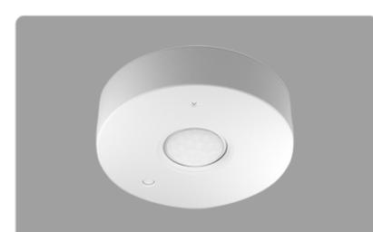
The Lightcloud Sensor is a dual-technology motion detector and closed loop daylight harvester that can switch and dim both local and remote circuits. It monitors power consumption, and can send an alert if power is lost. The Sensor is available for both standard and high bay applications, each with the option of surface or fixture mounting
