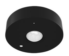
The Lightcloud Sensor is a dual-technology motion detector and closed loop daylight harvester that can switch and dim both local and remote circuits. It monitors power consumption, and can send an alert if power is lost. The Sensor is available for both standard and high bay applications, each with the option of surface or fixture mounting.
