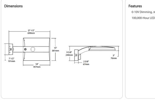
0-10V Dimming, standard 100,000-Hour LED lifespan
