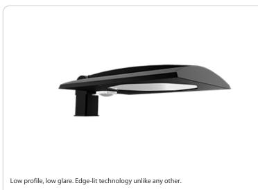
**Project:** Type: Prepared By: Date: **LED Info Driver Info Constant Current** Watts 117W Туре 120V 1.00A Color Temp 5000K (Cool) 208V 0.58A Color Accuracy 75 CRI 240V 0.50A L70 Lifespan 100,000 Hours 277V 0.43A Lumens 14,322 lm
